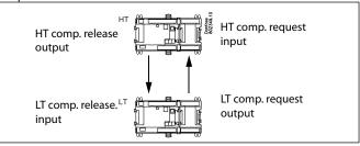
Here both a relay output and an On/off input are used on both controllers.
