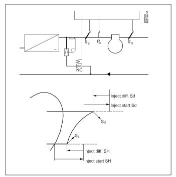
The high-pressure gas temperature can be kept down by means of liquid injection into the suction line.
