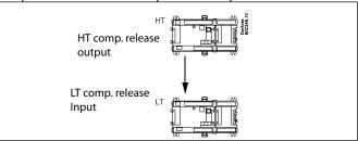
When a compressor is running in the high-pressure circuit, the controller will also pull the relay with the release signal into the low-pressure circuit.
