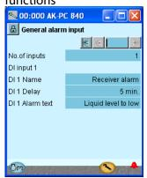
In our example we select one alarm function for monitoring the liquid level in the receiver. We have subsequently selected a name for the alarm function and for the alarm text.
