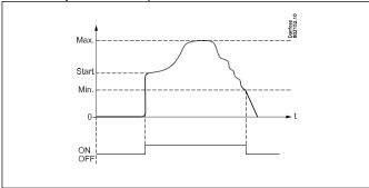
The speed-controlled compressor will always be the first to start and the last to stop. The frequency converter will be started when a capacity requirement corresponding to the mentioned "Start speed" arises (the relay output changes to ON and the analog output is supplied with a voltage corresponding to this speed). It is now up to the frequency converter to bring the speed up to "Start speed".
