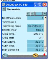
In our example we select one thermostat function for monitoring the plant room temperature.
