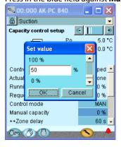
If you need to manually adjust the capacity of the compressors, you can use the following procedure:
