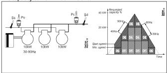
As the variable part of the speed controlled compressor is bigger than the following compressor steps, the capacity curve will be without holes.
