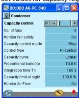
pressure is controlled on the basis of the outdoor temperature (floating reference). The settings shown here in the
