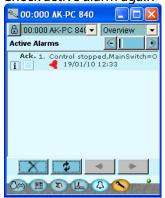
In our case an active alarm remains because the control has stopped. This alarm must be active when control has not started. We are now ready for the startup of control.
