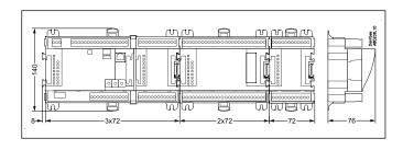
Example continued: Controller module + 1 extension module in 100-series = 224 + 72 = 296 mm.
