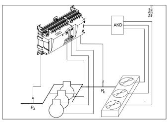
The controller's main function is to control compressors and condensers so that operation all the time takes place at the energy-optimum pressure conditions. Both suction pressure and condensing pressure are controlled by signals from pressure transmitters.
