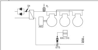
When the controlling sensor is selected as S4, P0 is used as a safety function for low suction pressure and will ensure disconnection of compressor capacity (frost protection).
