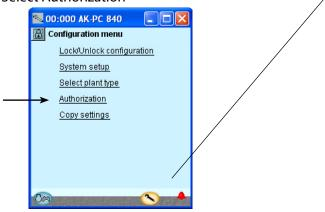
When the controller is supplied it has been set with standard authorization for different user interfaces. This setting should be changed and adapted to the plant. The changes can be made now or later.
