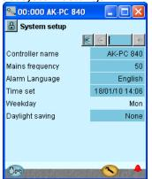
All system settings can be changed by pressing in the blue field with the setting and then indicating the value of the required setting.
