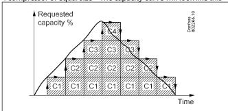
Cut-out of the last compressor stage:
